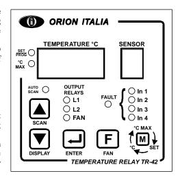
**FAN BUTTON:** it allows to switch between "always ON" or Automatic Fan Operation. In "always ON" mode, the Fan will be always ON and the led FAN will be ON.
