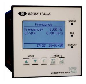
The device has been designed for continuous monitoring of the system's voltage, frequency and related variations. It is able to disconnect one or more loads in case of underfrequency (up to 7 stages) or frequency negative rate of change (up to 2 stages).
